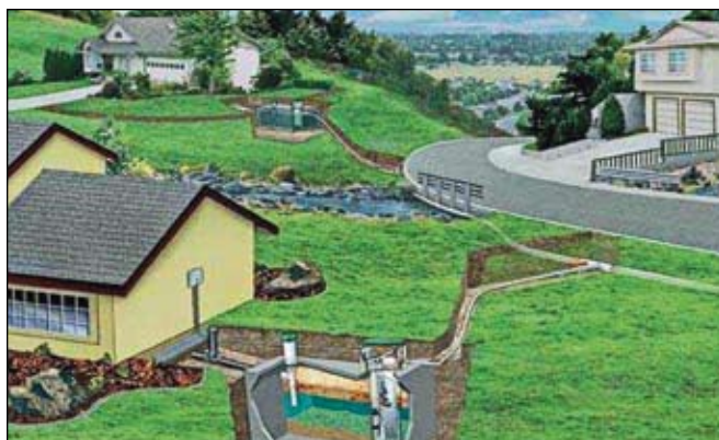
Fig 7: Septic Tank Effluent Pump. Source: Orenco Systems, Inc.
