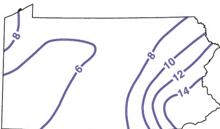
Figure 3. An earthquake-hazard map for Pennsylvania. The contours represent earthquake ground motions that have a 2 percent probability of being experienced in 50 years. The numbers are percentages of g , the acceleration due to gravity. See Table 3 for approximate corresponding values of Modified Mercalli intensity. From Frankel and others (2002).
