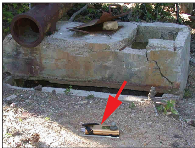
Figure 4—A radioisotope device (arrow) being used to check for heavy metals in the soil.
